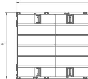
100MM Bearer Model Length: 229" Width: 89" Height: 6" Weight: 1700 LBS Capacity: 15 Tons Return: 20 Per 20' Container
